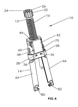
Figure 4 is an isometric view of the rod reducing device with the screw jack mechanism fully retracted and the two elongated grasping members in an open configuration. Ex. 1201, 3:2–32.
